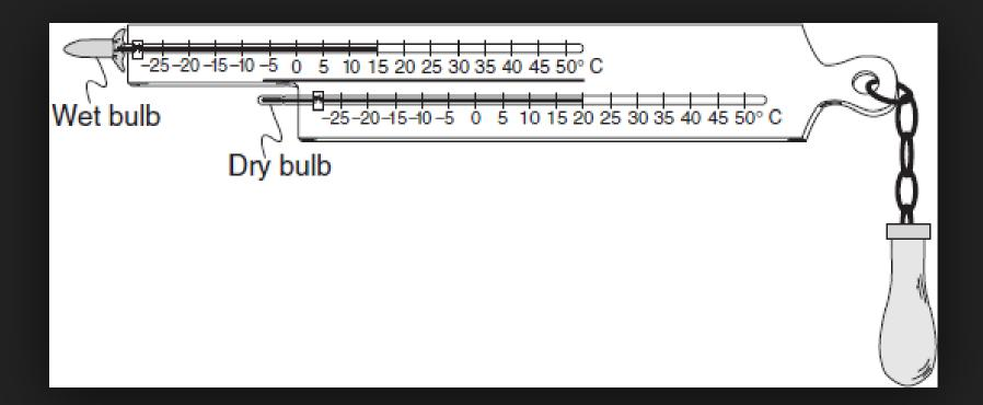
Wet-bulb temperature (WBT) is affected by the moisture content of the air (evaporative cooling)
