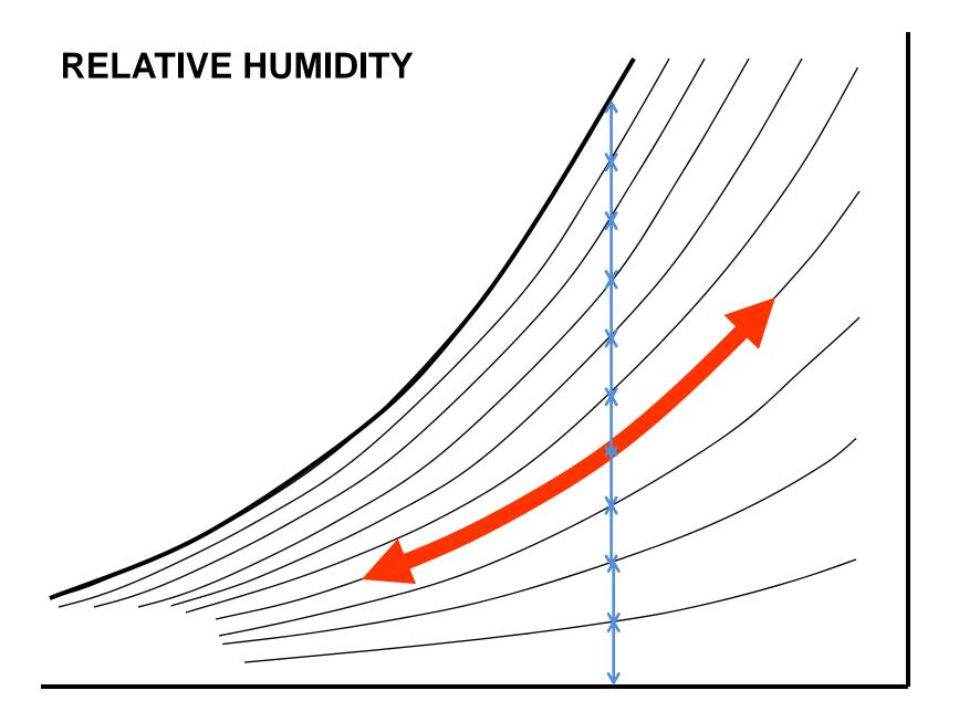
Knowing any two of these properties of a sample of air (DBT, WBT, RH, MC, dew point or saturation temperature), the other properties can be determined with the Psychrometric Chart
